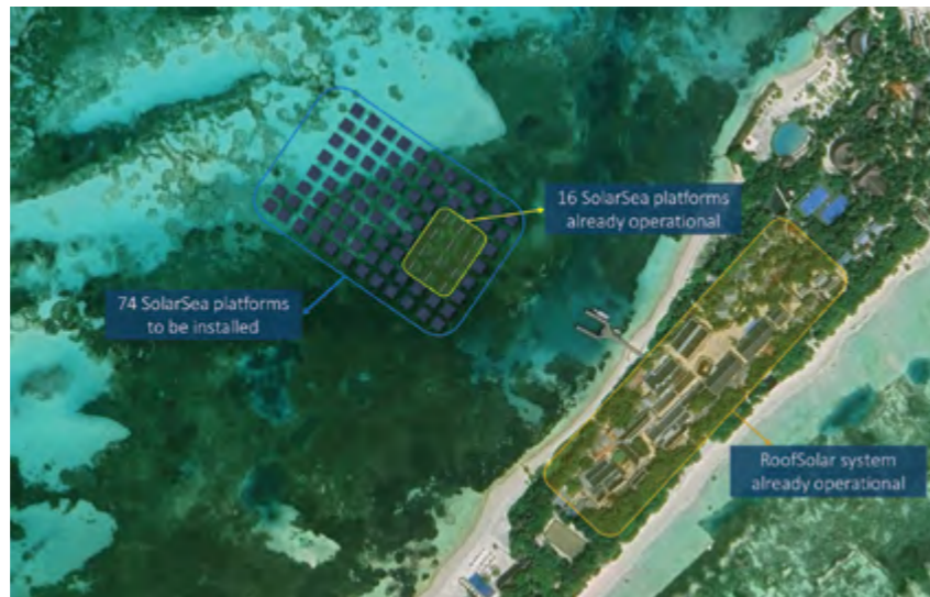
A look at the preliminary layout: The existing system is planned to be expanded to 90 floating solar platforms.
